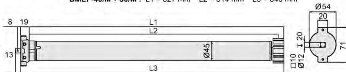
**Standard-Motor kurz** : DM-10-K : L1 = 345 mm L2 = 320 mm L3 = 360 mm
