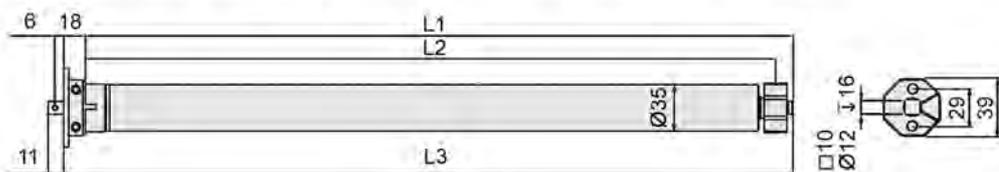
**Mini-Elektronikmotor** : ME-10/40 : L1 = 567 mm L2 = 553 mm L3 = 585 mm
