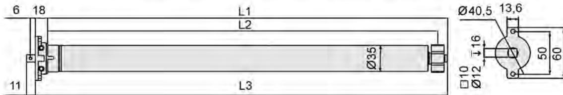
**Mini-Motor kurz** : DM-10/40-K : L1 = 377 mm L2 = 362 mm L3 = 395 mm
